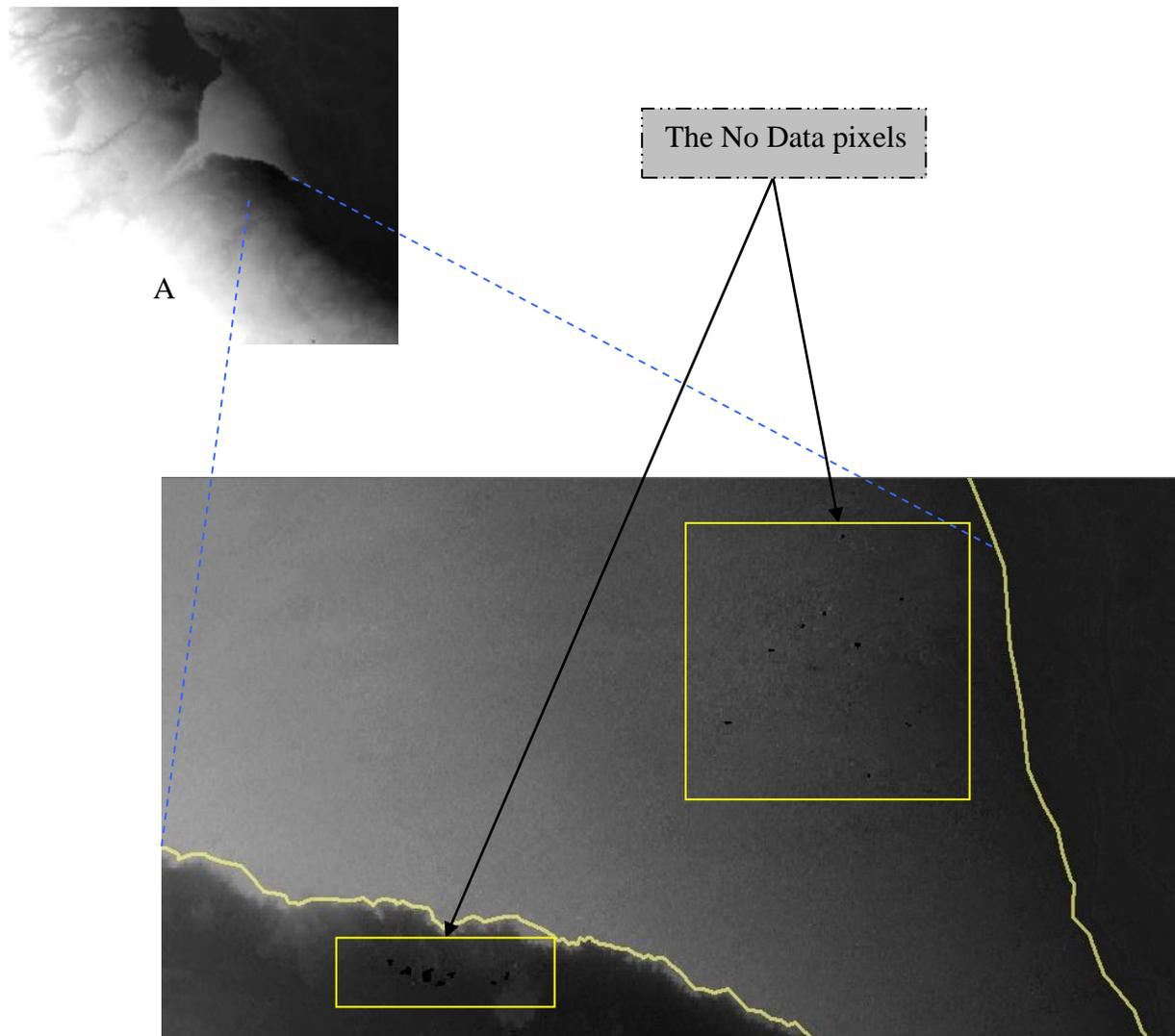
**Figure 3-** A) the original 30m SRTM Digital Elevation Model mosaic image with its No Data pixels image illustrated bellow.
