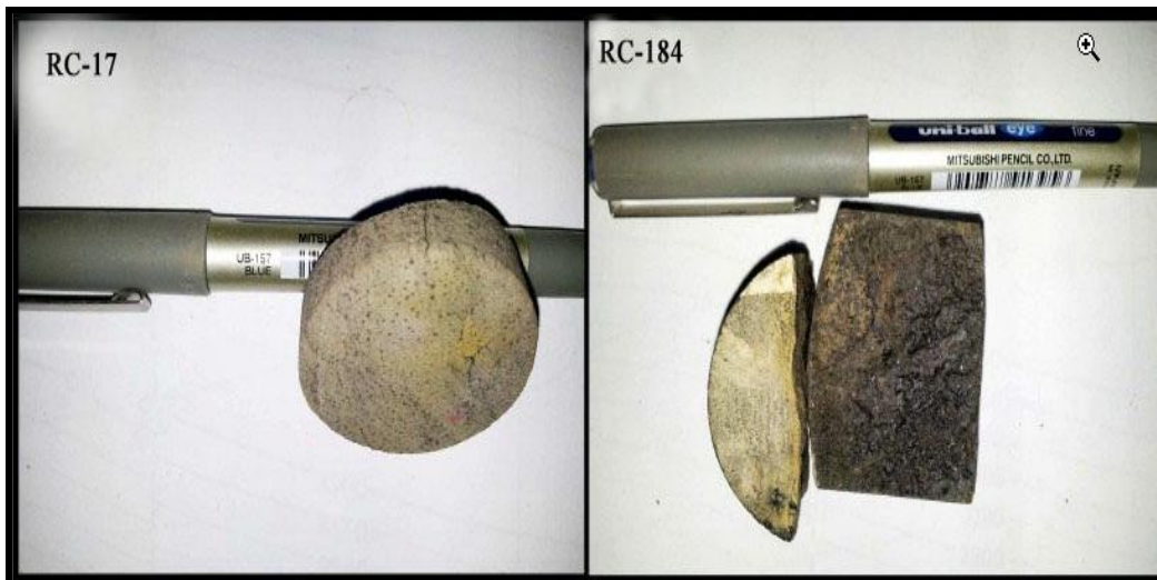
Plate 1- Core Sample (RC-17, Depth = 3157m), (RC-184, Depth = 3199m) collected from the Zubair Formation in North Rumaila Field
